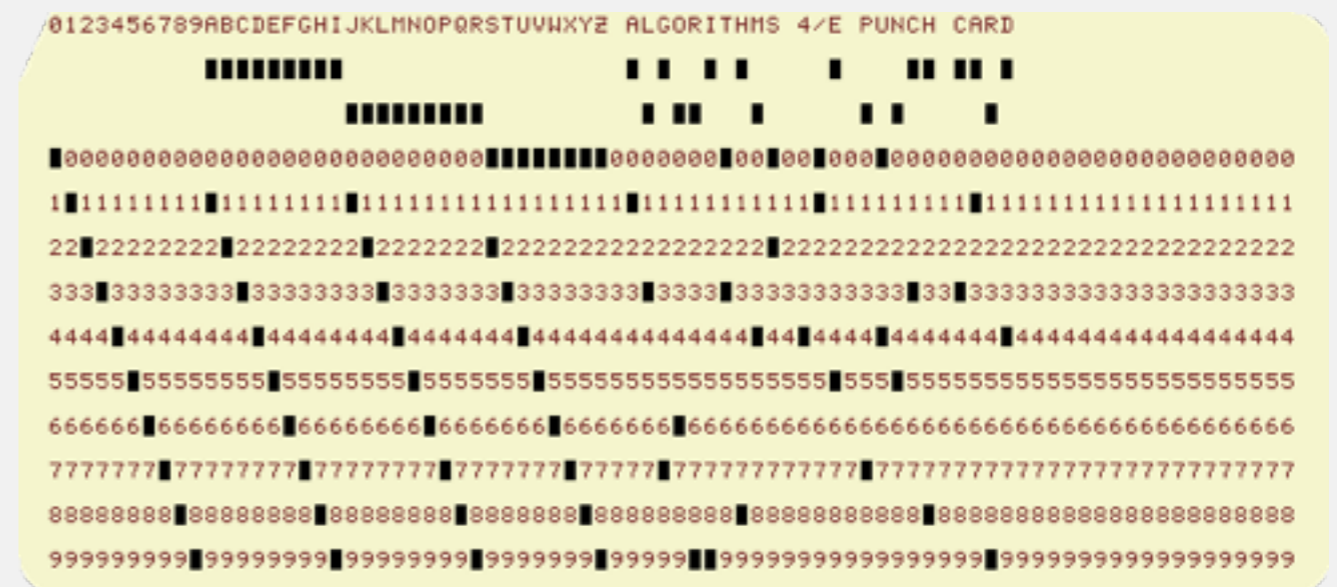
punch card (12 holes per column)
