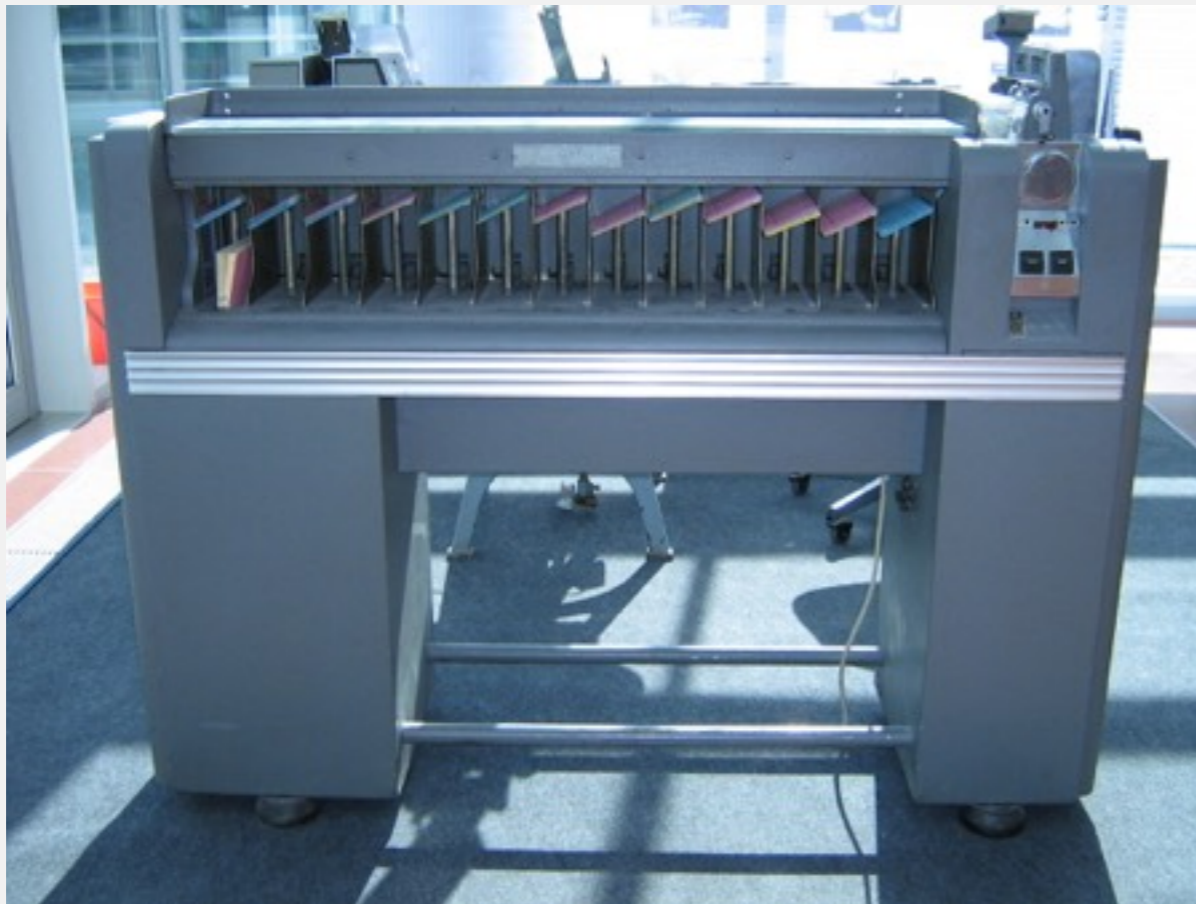
IBM 80 Series Card Sorter (650 cards per minute)
