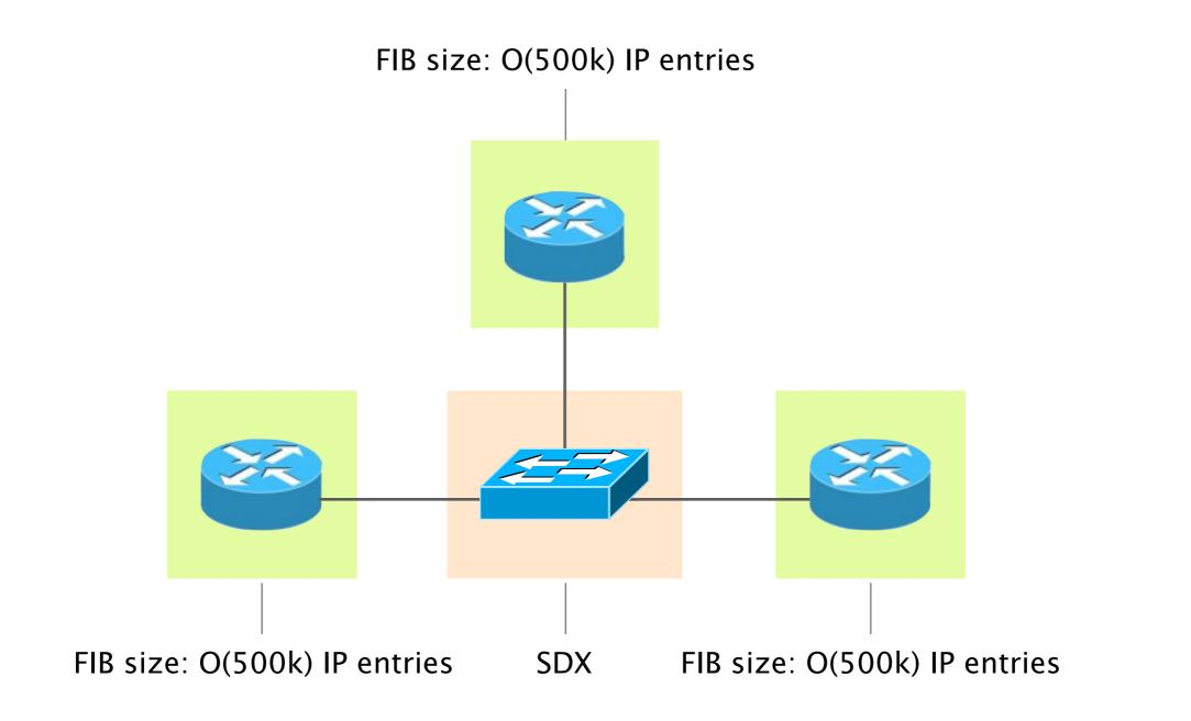
SDX considers edge routers' FIB as the first stage of a multi-stage FIB
