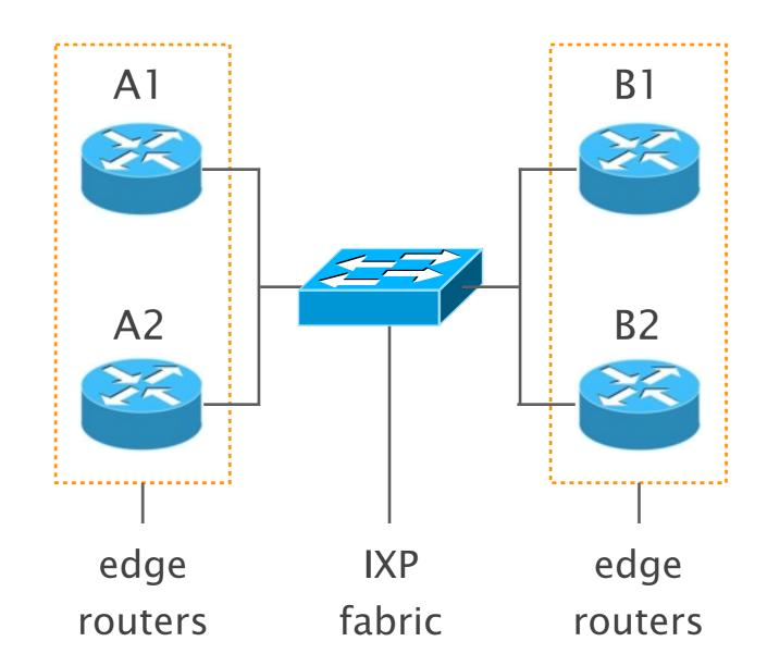
Router B2 is a backup router, it may be used only upon B1's failure
