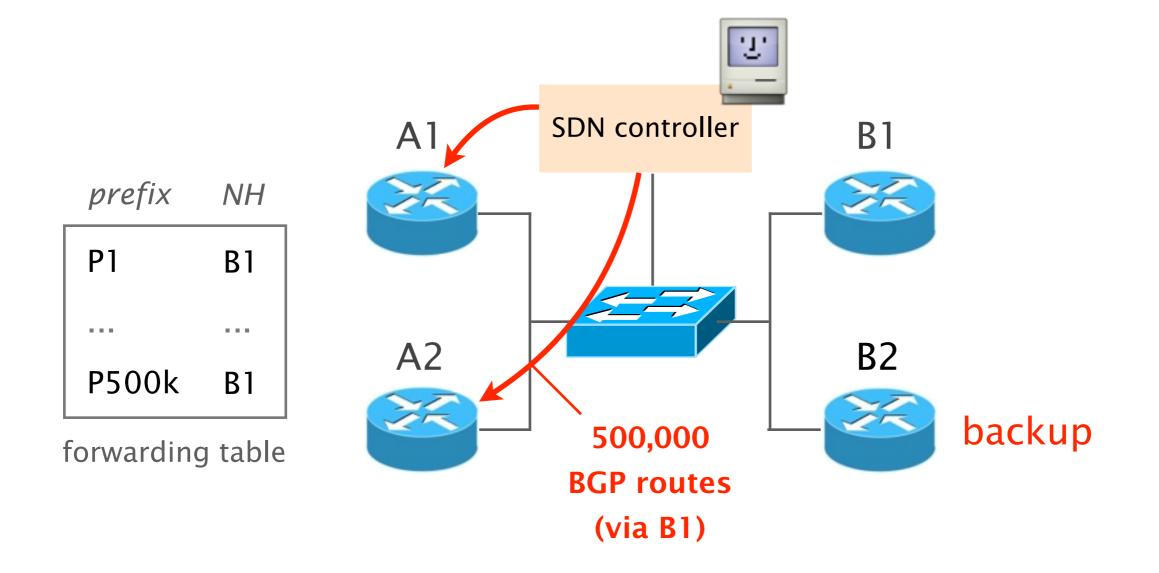
Upon a peer failure, the SDX controller directly pushes next-hop rewrite rules
