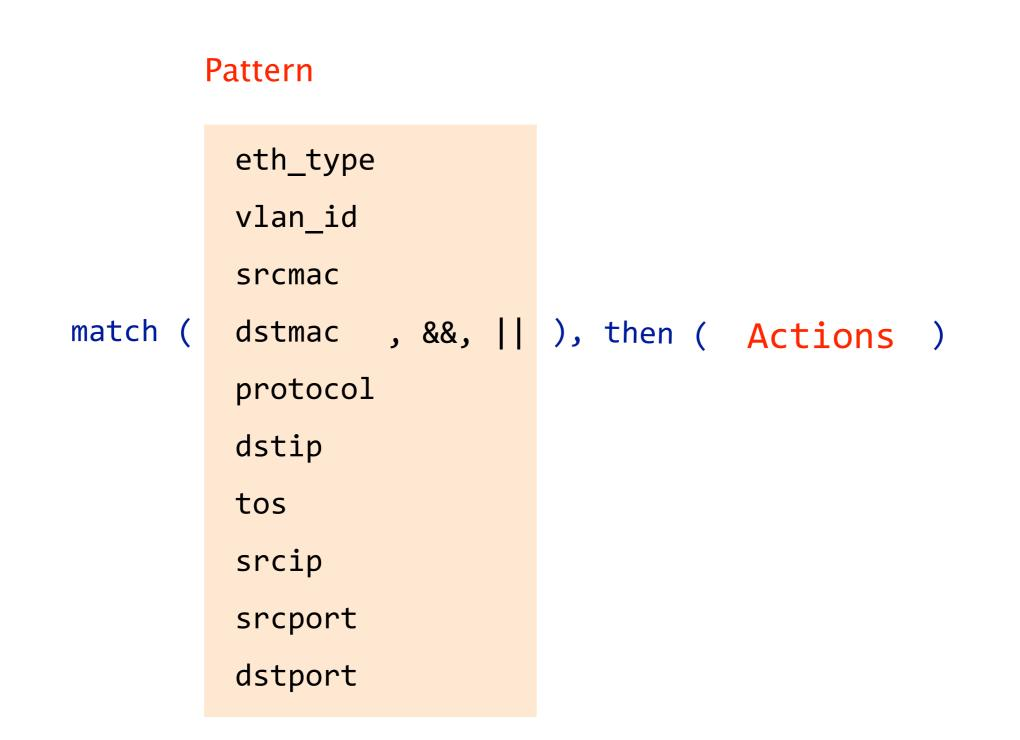
Pattern selects packets based on any header fields, while actions forward or modify the selected packets
