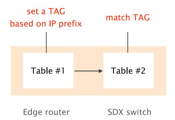
SDX uses BGP NH as a provisioning interface and MAC addresses as tag in the data-plane
