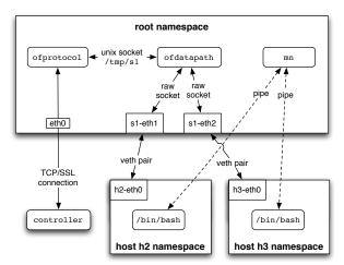
Figure 1: Mininet creates a virtual network by placing host processes in network namespaces and connecting them with virtual Ethernet (veth) pairs. In this example, they connect to a userspace OpenFlow switch.
