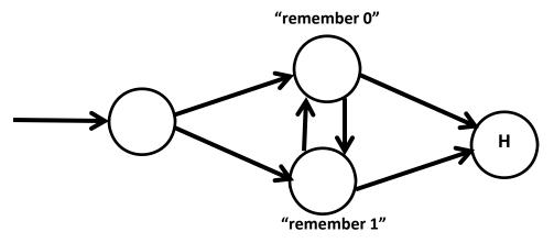
6. (Bonus) Complete the following TM so that it accepts well-formed balanced parenthesis expressions like (()()) or ((())) and rejects badly-formed ones like (() or )(. Assume it starts on the left edge of the input. You have to determine the new target of each transition.
