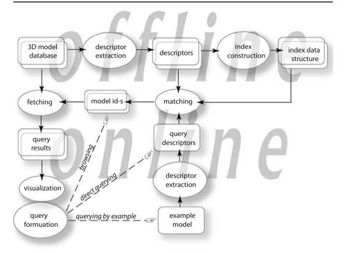
Fig. 1 Conceptual framework for shape retrieval
