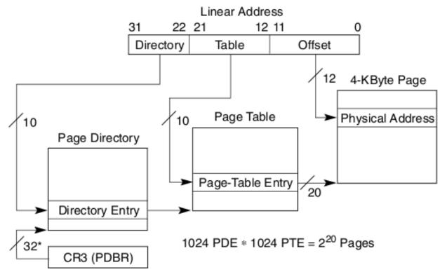
\*32 bits aligned onto a 4-KByte boundary.
