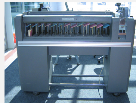
IBM 80 Series Card Sorter (650 cards per minute)
