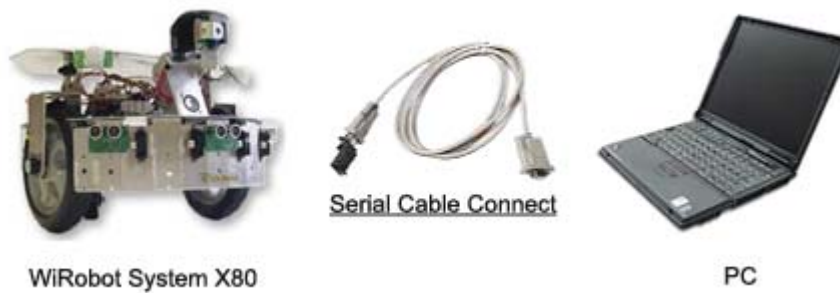
Figure IV.3 WiRobot System Setup without Wireless Connection
