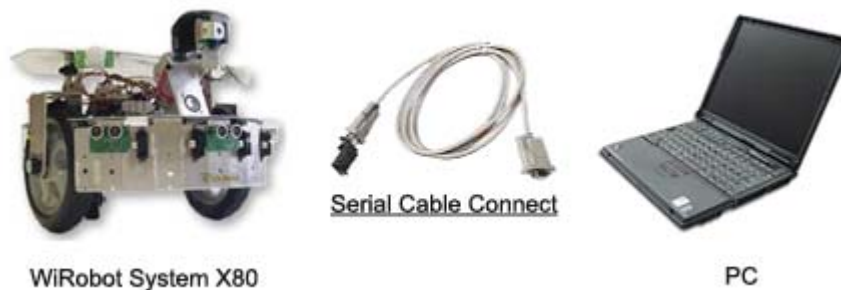
Figure IV.3 WiRobot System Setup without Wireless Connection
