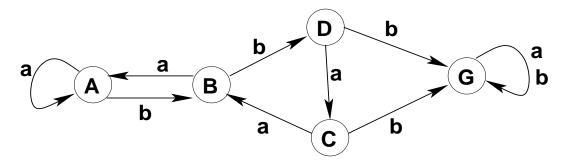
There are five states: A, B, C, D and G. The reward at every state is -1, except at G where the reward is 0. There are two actions, a and b, and the effect of each action is deterministic as indicated in the figure. For instance, executing a in state B leads to state A. Assume  $\gamma = 1$  in this problem.
