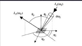
Figure 2.9: Bidirectional reflection distribution function.
