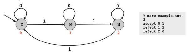
The first line of example.txt gives the number of states N. The state names are numbers from 0 to N-1. Subsequent lines of example.txt give the state types and the transitions (the ith line describes state i): each line has accept or reject followed by two state names, the first giving the transition if the input is 0 and the second giving the transition if the input is 1. Assume that the start state is always state 0.
