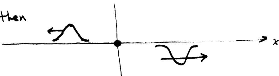
$\therefore$  wave shape is inverted on reflection from fixed end.
