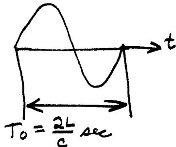
$$f_0 = \frac{1}{T_0} = \frac{c}{2L} \text{ Hz (cycles/sec)}$$
