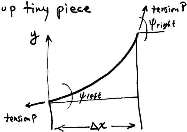
$$\text{net vertical component of force on segment} = P \sin \psi_{\text{right}} - P \sin \psi_{\text{left}} = m a = \underbrace{\cancel{P} \Delta x}_{\text{mass}} \frac{\partial^2 y}{\partial t^2}$$
