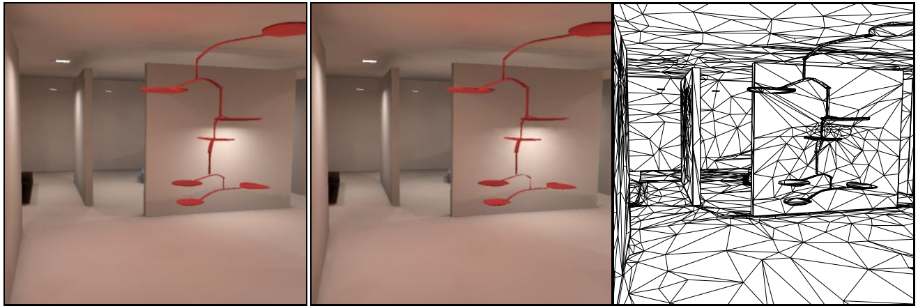
Figure 11: Simplification of a radiosity solution; left: original mesh (150,983 faces); right: simplified mesh (10,000 faces).
