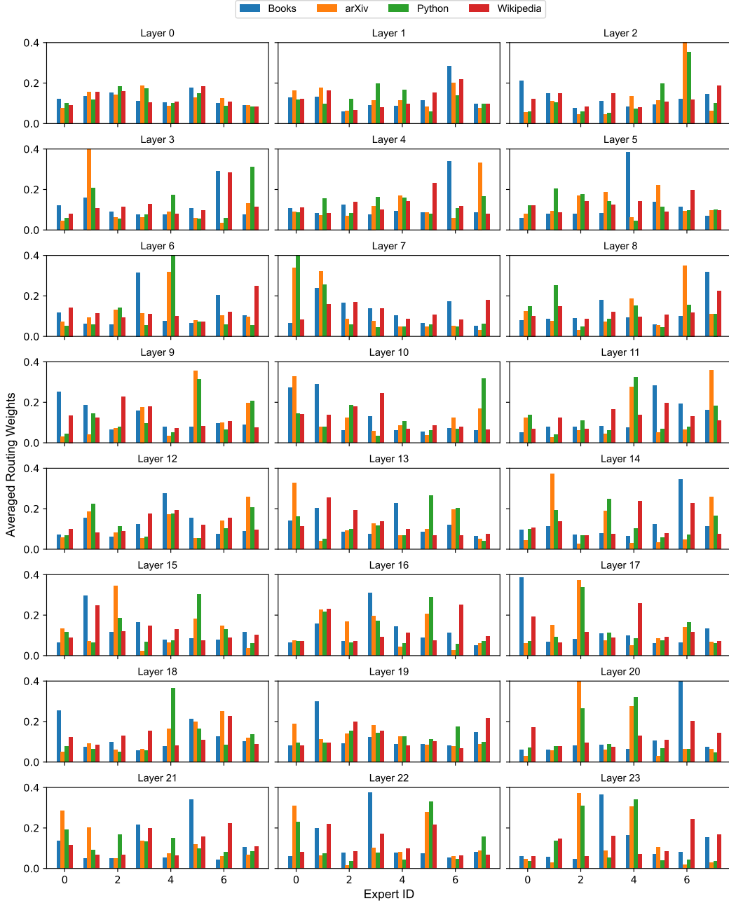
Figure 12: Averaged routing weights at all the layer of the 0.3B/8E model on different domains (Books, arXiv, Python, Wikipedia). We observe that the experts in our MoE models learn clear domain-level specialization.
