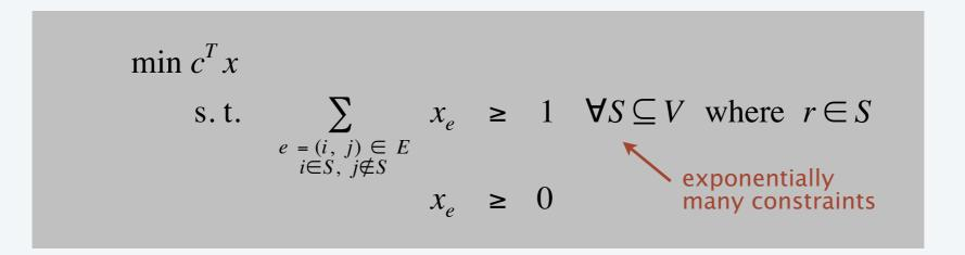
Separation oracle. Perform at most n - 1 min cut procedures with r as the source and edge weights  $x_e$ .
