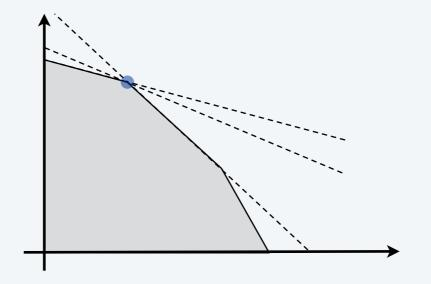
Cycling. Infinite loop by cycling through different bases that all correspond to same vertex.
