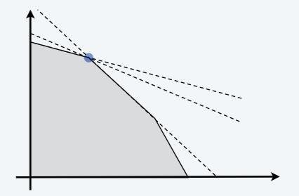
**Degenerate pivot.** Min ratio = 0.
