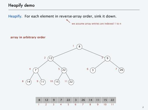
Heapify. For each element in reverse-array order, sink it down.
