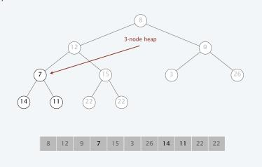
Heapify. For each element in reverse-array order, sink it down.
