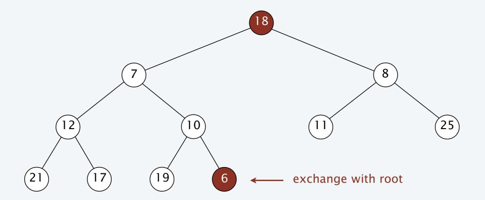
Extract min. Exchange root node with last node; repeatedly exchange element in parent with element in larger child until heap order is restored.
