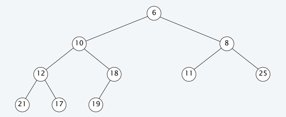
Insert. Add node at end; repeatedly exchange element in child with element in parent until heap order is restored.
