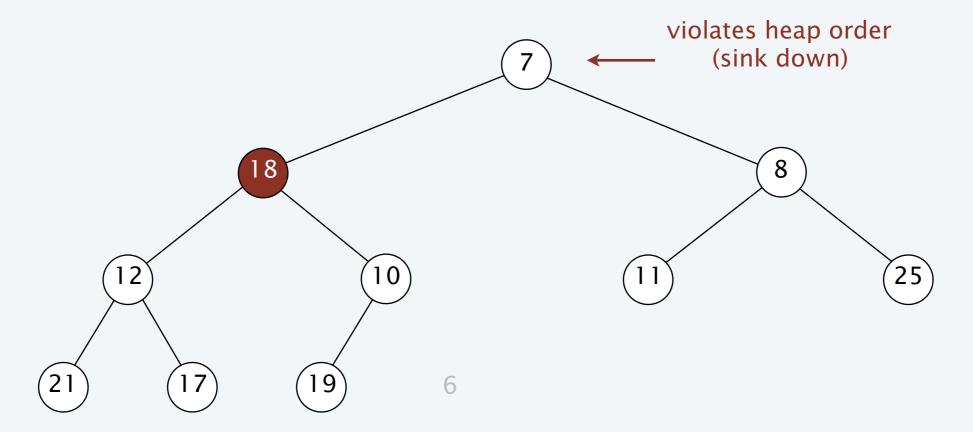
Extract min. Exchange root node with last node; repeatedly exchange element in parent with element in larger child until heap order is restored.
