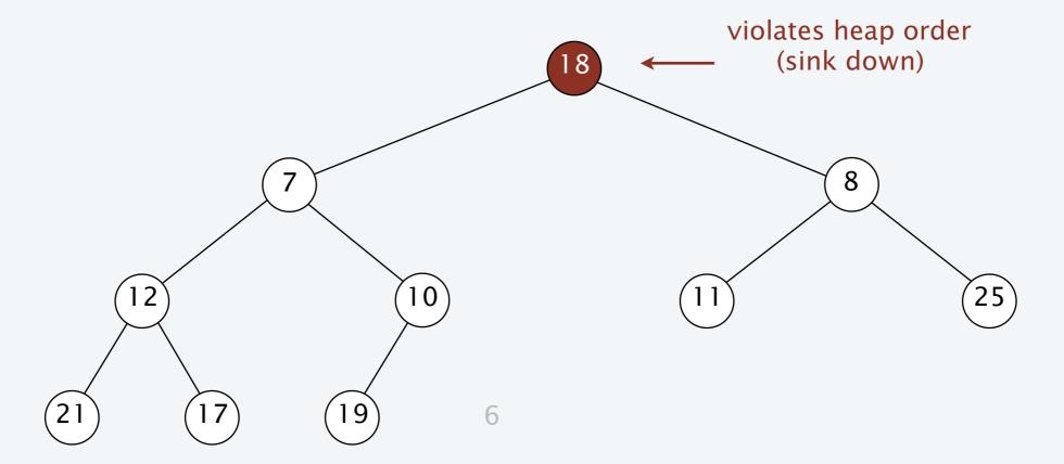
Extract min. Exchange root node with last node; repeatedly exchange element in parent with element in larger child until heap order is restored.
