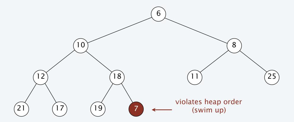
Insert. Add node at end; repeatedly exchange element in child with element in parent until heap order is restored.
