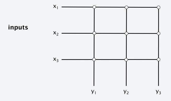
FIFO queueing. Each input *x* maintains one queue of cells to be routed.
