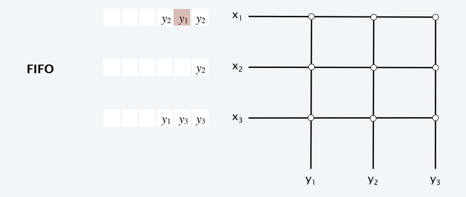
FIFO queueing. Each input *x* maintains one queue of cells to be routed.
