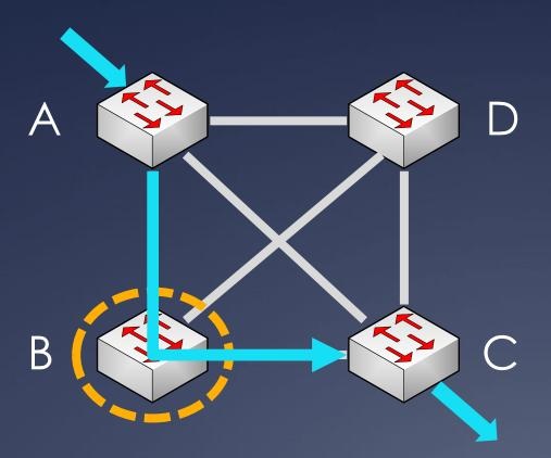
TE writes new value of routing state of B for tunneling traffic
