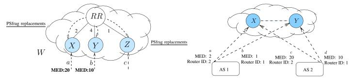
Fig. 6. When an AS's iBGP topology uses route reflectors and MED, a router may not always select a route in  $\gamma(E)$ .
