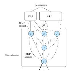
Fig. 1. Network with three egress routers connecting to two neighboring ASes: Solid lines correspond to physical links (internal links are annotated with IGP link weights) and dashed lines correspond to BGP sessions. Thick lines illustrate the shortest path from one router to its closest egress point for reaching the destination.
