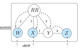
Fig. 12. When an AS's iBGP topology uses route reflectors, a router may not always discover the route corresponding to its closest egress router.
