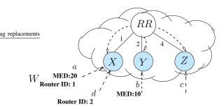
(b) When X is closer to RR than Y, the routing system violates safety and the algorithm in Figure 13 is incorrect.
