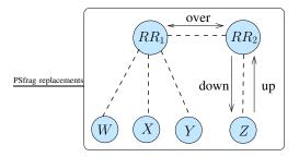
Fig. 11. Example iBGP signaling graph.
