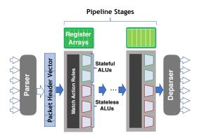
Figure 2: Protocol Independent Switch Architecture (PISA)
