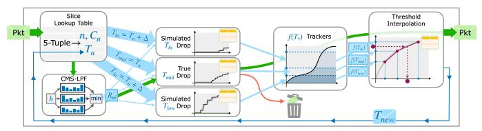
Fig. 3. When a packet arrives, AHAB first maps it to a slice n and estimates its user's sending rate  $R_m$  using the CMS-LPF estimator (§IV-B), then uses probabilistic dropping to enforce slice n's bandwidth limit  $T_n$  (§V-A). AHAB also maintains two bandwidth limit candidates  $T_{low}$ ,  $T_{hi}$  and tracks the hypothetical total bandwidth usage  $f(\cdot)$  (§V-B), which is used to derive a more accurate bandwidth limit  $T_{new}$  via approximated linear interpolation (§V-C).
