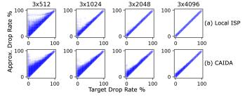
Fig. 12. 3x4096 CMS-LPF estimator is sufficient for serving millions of users, with negligible error in drop probability.
