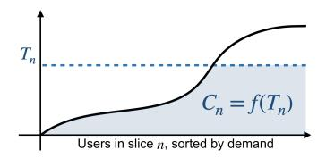
Fig. 1. We calculate and enforce per-user bandwidth limit  $T_n$  for all users in slice n, so that their total bandwidth consumed is equal to capacity  $C_n$ .
