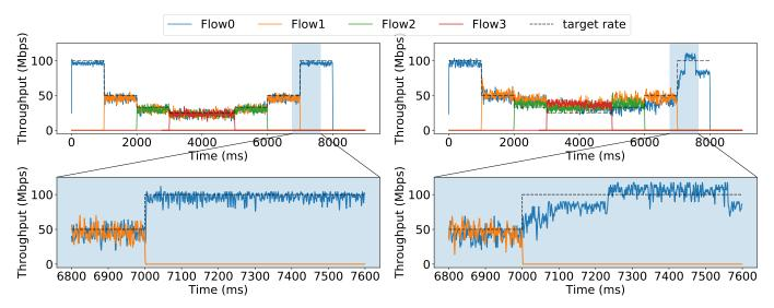
Fig. 7. AHAB (left) converges to fair bandwidth allocation within 3.1ms on average, while HCSFQ [21] (right) needs 42.3ms.
