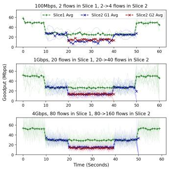
Fig. 11. Three experiments showing two slices sharing a common bottleneck. Slice 1 uses half the bandwidth even when Slice 2 has twice as many flows.
