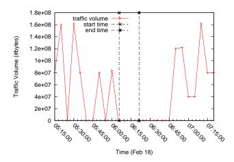
Figure 4: After the BGP withdrawal, the IP addresses matched a less-specific prefix; still, no traffic to these destination IP addresses was observed until after the more-specific prefix was announced again (Feb 18, 2009).
