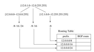
Figure 2: Storing address ranges and prefix sets for prefixes 12/8, 12/16, and 12/24
