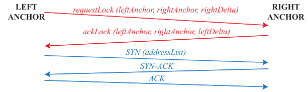
Fig. 4. Control packets exchanged for reconfiguration. Red packets travel on the old path, blue on the new path.
