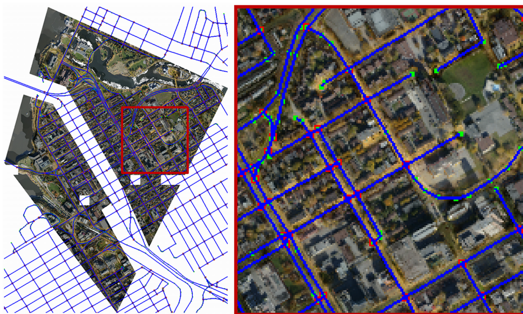
Figure 3: Open Street Map data provided as input to our method (OpenStreetMap, 2010). Zoomed view of area highlighted with red rectangle appears on right. Red points are intersections. Green points are polyline vertices. Blue lines are roads.
