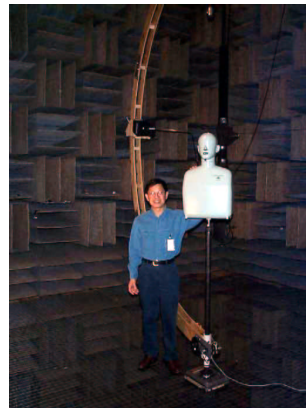
Figure 24: HRTF measurement setup in Bell Labs' anechoic chamber.
