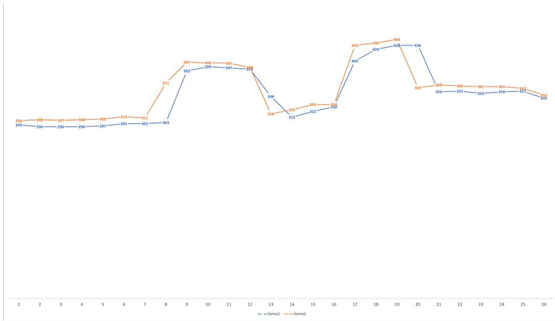
Figure 3. Plot graph of sensor data points when the robot was passing two doors in a row. Y-axis represents distance from sensor, in mm, X-axis represents time, with the time interval being 0.25 seconds. Series 1 represents sensor 0, the farthest back right. Series 2 is sensor 1, the front right.
