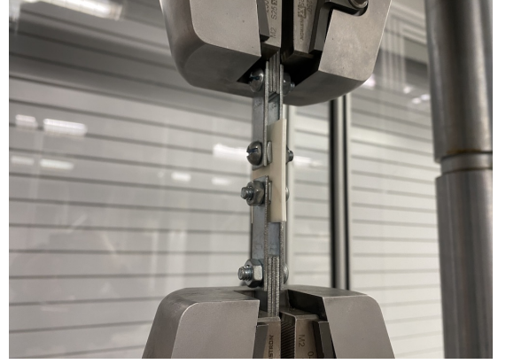
Figure 3: A 3D printed part being tested on a universal testing machine (Instron 600DX), with square nuts in the trapezoidal holes. The machine moves at a speed of 20 mm/min and stops when the object breaks or by a manual stop.
