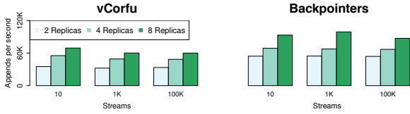
Figure 7: vCorfu’s replication protocol imposes a small penalty on writes to support materialization. Each run is denoted with the number of streams used.
