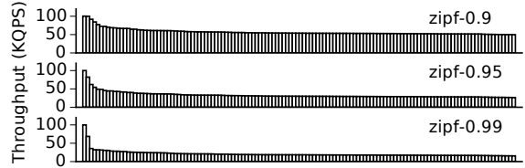
Figure 9: Throughput of each backend node without cache under workloads with different Zipf skewness. Node IDs (x-axis) are sorted according to their throughput.
