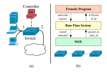
Figure 2. (a) Simple network topology (b) Frenetic architecture
