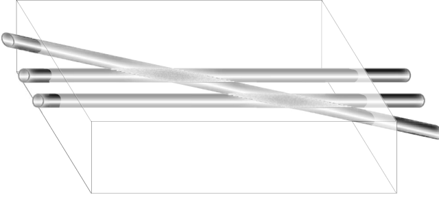
FIGURE 1 Possible soliton computing device in which spatial solitons interact in a nonlinear medium.
