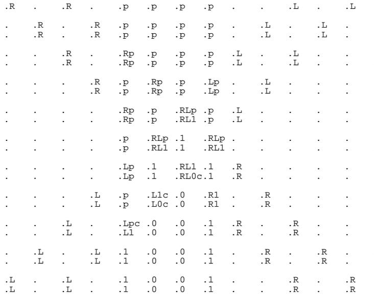
**Fig. 1.5** Simulator output for PM multiplication. The top line in the figure gives the initial state of the PM’s medium, representing the multiplication problem  $11_2 * 11_2$ , as described in the text. Each successive pair of lines depicts the state of the medium after the propagation and collision phases of each time step. The bottom line in the picture shows the stationary answer,  $1001_2$ , in the central computation region, along with the unchanged operands moving away from the region.
