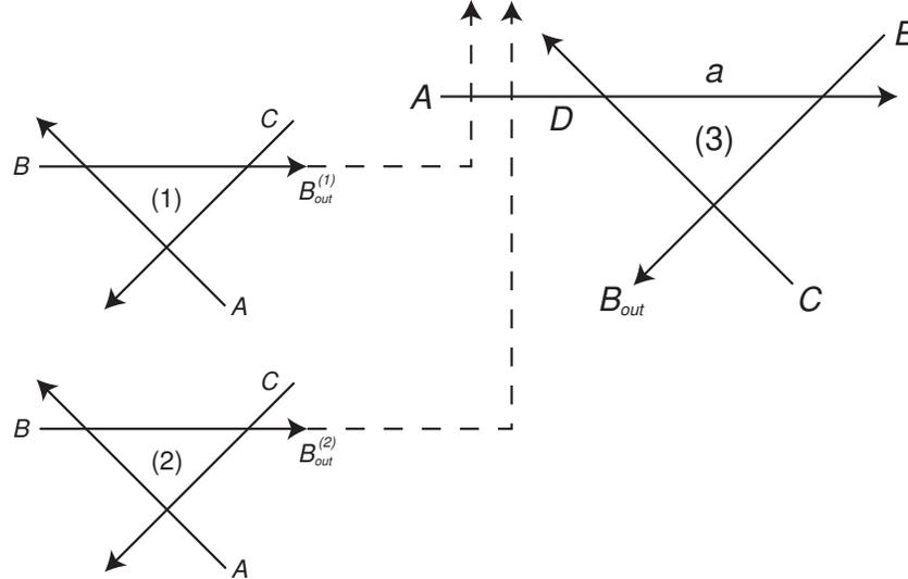
**Fig. 1.25** Schematic of NAND gate using bistable collision cycles.
