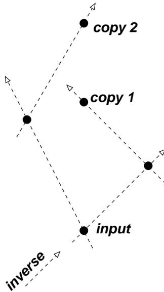
**Fig. 1.20** The introduction of a second speed makes true FANOUT possible. For simplicity data and operator pulses are indicated by solid dots, and the  $y$  operator pulses are not shown. The paths of actuator pulses are indicated by dashed lines.
