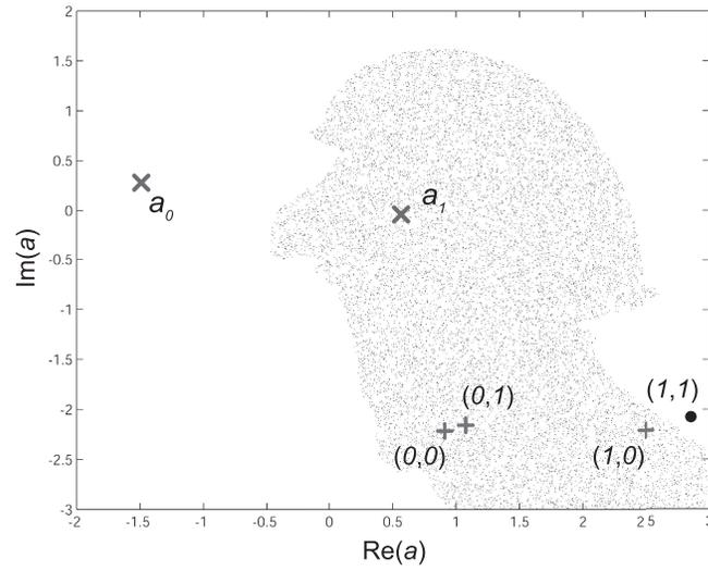
**Fig. 1.26** Map of beam  $a$  in the complex plane showing NAND gate operation. The two foci,  $a_0$  and  $a_1$ , are shown with their corresponding basins of attraction. The + signs are monostable foci which indicate inputs where the cycle reaches state 1, the • is the monostable focus acquired with a (1, 1) input.
