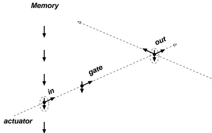
**Fig. 1.19** The frame of this figure is moving down with the data pulses on the left. A data pulse in memory is operated on with a three-collision gate actuated from the left, and the result deposited to the upper right.
