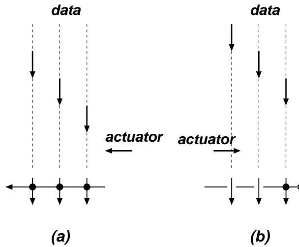
**Fig. 1.18** (a) When entered from the right and properly timed, the actuator pulse hits all three data pulses, as indicated in the projection at the bottom; (b) When entered from the left and properly timed, the actuator pulse misses two data pulses and hits only the rightmost data pulse, as indicated in the projection at the bottom.
