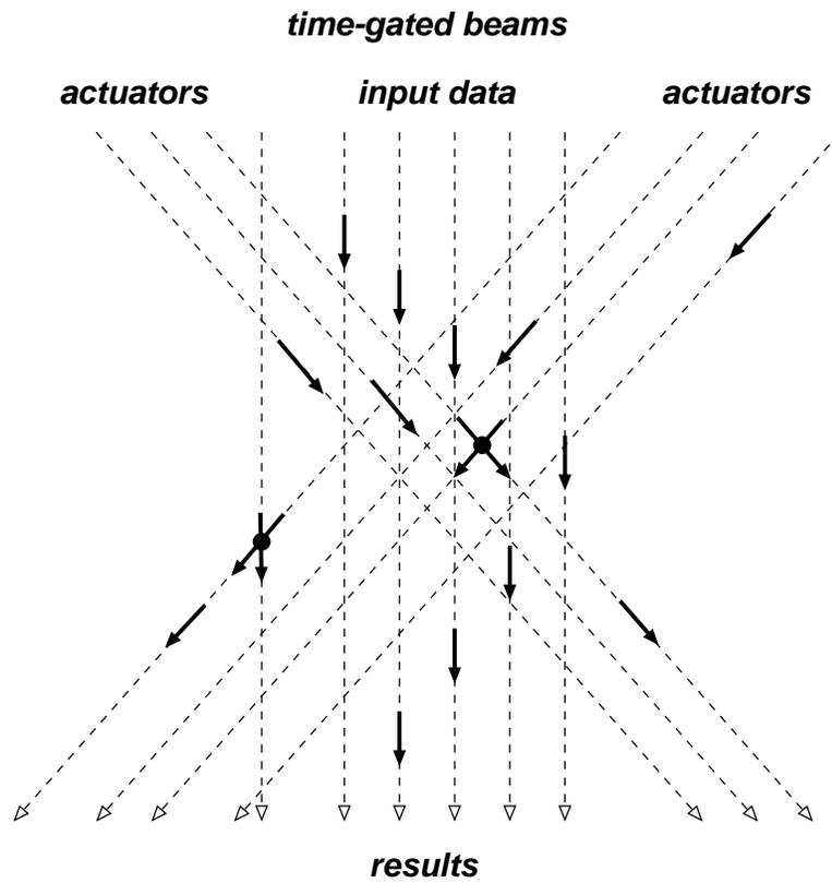
**Fig. 1.12** The general physical arrangement considered in the construction of a universal collision-based computer. Time-gated beams of spatial Manakov solitons enter at the top of the medium, and their collisions result in state changes that reflect computation. Each solid arrow represents a beam segment in a particular state.
