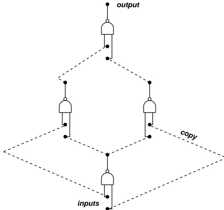
**Fig. 1.21** Implementation of an XOR gate with NAND gates and COPY operations. The results are deposited above the inputs in the data column. Two speeds are necessary to achieve the fanout.
