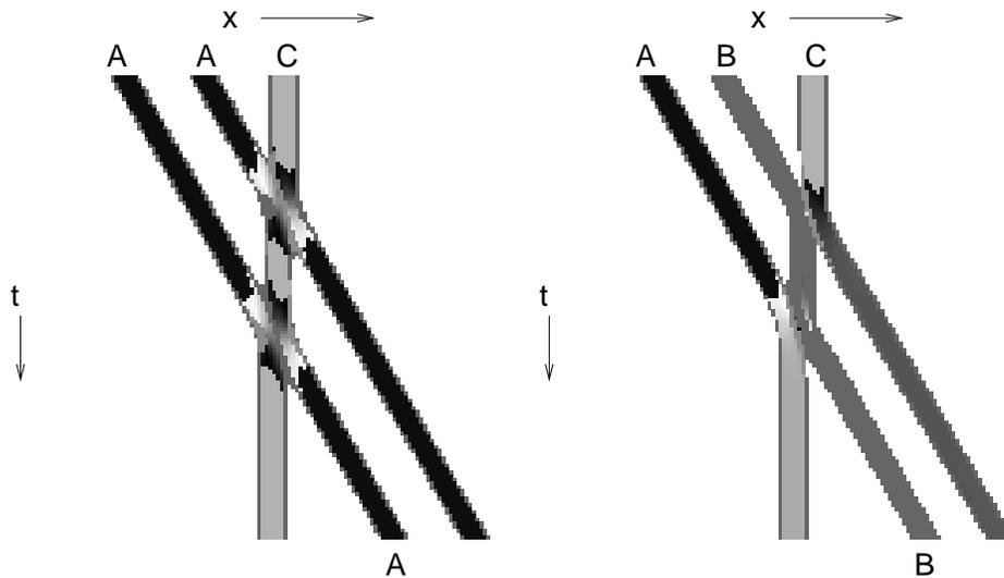
**Fig. 1.11** Numerical simulation of a "move" operation implemented in the Manakov system. These graphs display the color-coded phase of  $\rho$ . In each graph, the information contained in the middle particle in the initial conditions (top of graphs) is moved to the middle particle in the final conditions (bottom of graphs). The information transfer is effected by the "carrier" particle  $C$ . These graphs were obtained by numerical simulation of Eq. 1.2 with  $\mu = 1$ .
