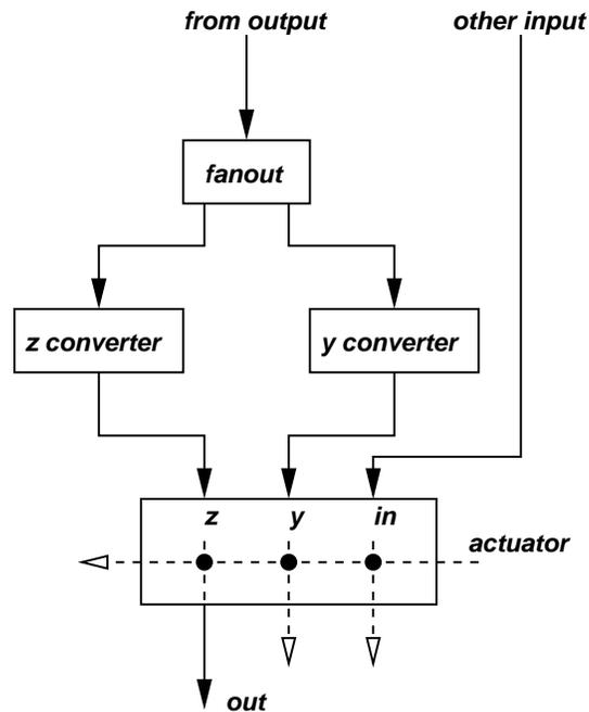
**Fig. 1.17** A NAND gate, using converter gates to couple copies of one of its inputs to its  $z$  and  $y$  parameters.
