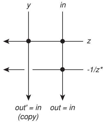
**Fig. 1.27** Schematic of FANOUT gate, where each • indicates a collision.
