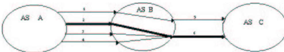
Fig. 2. AS A sending traffic via AS B to destinations in AS C
