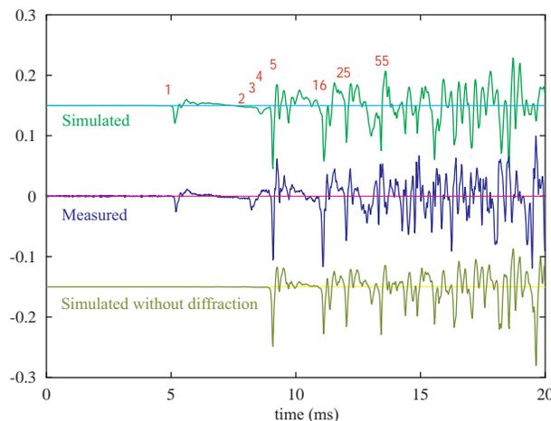
Figure 28: Comparison of the early part of a simulated and measured impulse response in the “Bell Labs Box”, a simple test environment. Some of the first 55 propagation paths are labeled on the top curve out of the 1300 simulated.
