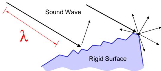
Figure 4: Sound waves impinging upon a surface usually reflect specularly and/or diffract at edges.
