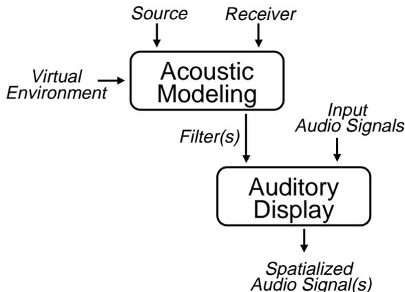
Figure 2: Basic auralization pipeline.
