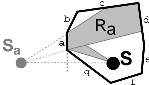
Figure 12: Beam tracing culls invisible virtual sources.
