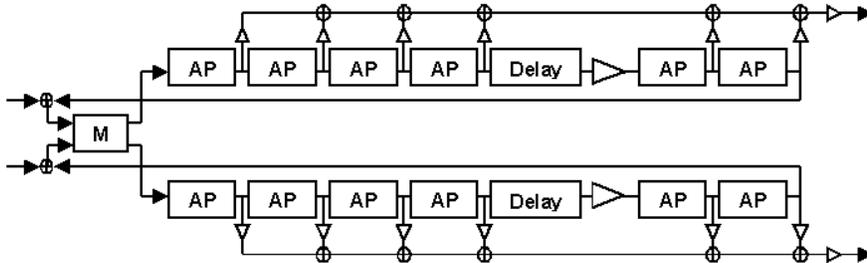
Figure 23: Example FDN reverberator based on cascaded all-pass filter chains.
