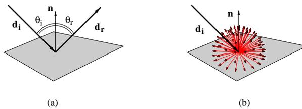
Figure 15: (a) specular reflection:  $\theta_r = \theta_i$ , (b) diffuse lambertian reflection.
