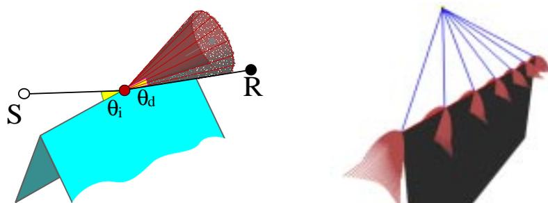
Figure 16: The Geometric Theory of Diffraction approximates diffraction of a ray incident to a wedge as a cone of diffracted rays, such that  $\theta_i = \theta_d$  (left). For each diffraction, a complex diffraction coefficient can be computed. Values of the UTD coefficients are visualized on the right for point-source radiating over a half-plane.
