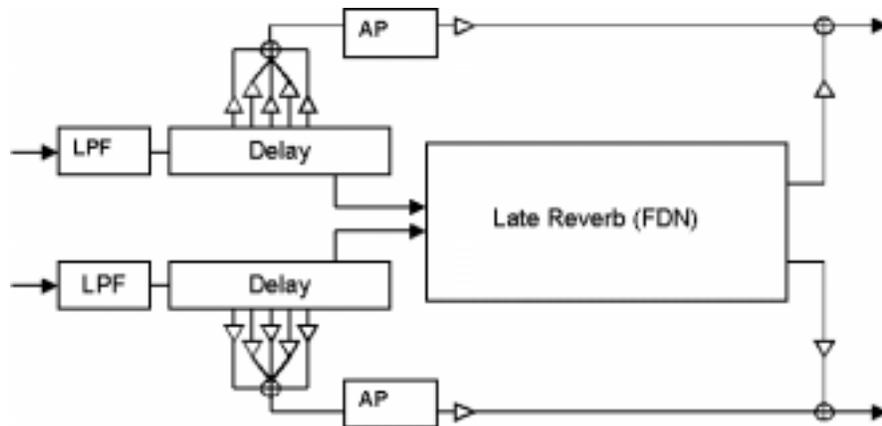
Figure 20: Example artificial reverberator.
