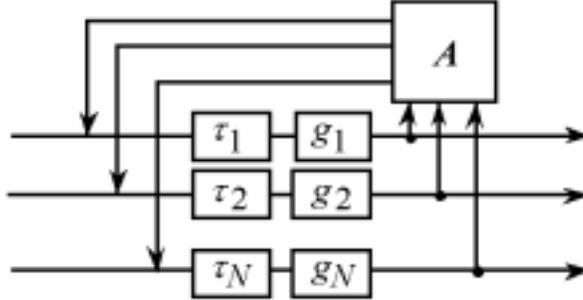
Figure 21: Basic feedback delay network.
