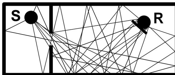
Figure 1: Sound propagation paths from a source (S) to a receiver (R).
