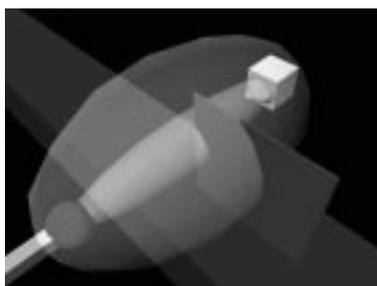
Figure 17: A 3D view of a virtual source (right), microphone (left), obstacles and first Fresnel ellipsoids computed at 400 and 1000 Hz. Occlusion ratio of the ellipsoids can be used to derive a frequency-dependent visibility factor [124].
