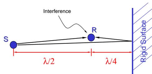
Figure 5: Interference can occur when two sound waves meet.
