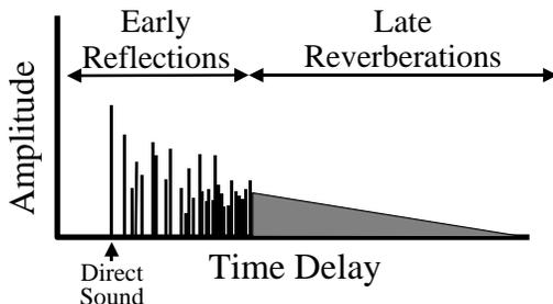
Figure 3: Direct, early, and late parts of an impulse response.
