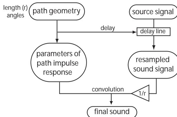
Figure 19: Signal processing pipeline for a sound path.
