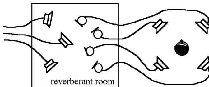
Figure 22: Conceptual analog of multi-channel reverberator simulating diffuse-field reverberation.
