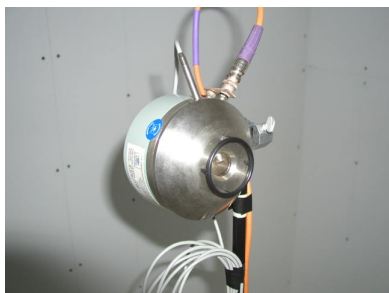
Figure 6: Our reference source, the Brüel&Kjaer artificial mouth .
