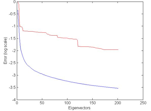
**Fig. 8:** Error in approximation of the biharmonic distance using the first  $K = 1, 2, \dots, 200$  eigenvectors is shown in log scale. The red curve demonstrated the maximum error and the blue curve the average error in approximating 200K pairwise distances randomly picked from a mesh with 5K vertices.
