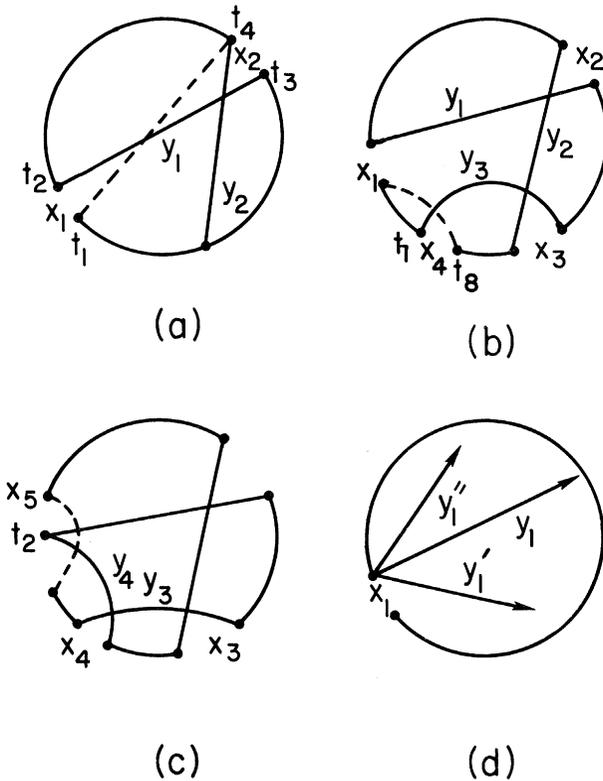
**Fig. 3.** Algorithm description, Step 4 (the dotted line indicates a possible close-up). (a)  $i=2$ . (b)  $i=4$ . Note that  $t_8$  is uniquely determined. (c)  $i=5$ . Note both original edges at  $t_5$  have been broken. (d) Backtracking in Step 6c: multiple choices for  $y_1$ .
