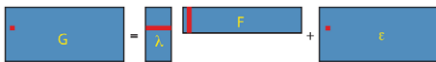
Figure 1. Low-dimensional matrix factorization via factor analysis. Each matrix in Equation 1 is illustrated by a blue rectangle and labeled. As in Equation 2, a single element of genotype matrix G , G_{i,j} is shown in red, and is computed from the product of the appropriate factor loading and factor vectors plus the corresponding random error term (all highlighted in red). doi:10.1371/journal.pgen.1001117.g001
