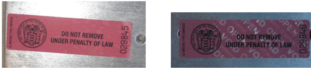
Figure 13: Pressure-sensitive adhesive tape. At left, as first installed; at right, when (mostly) peeled back and pressed down again
