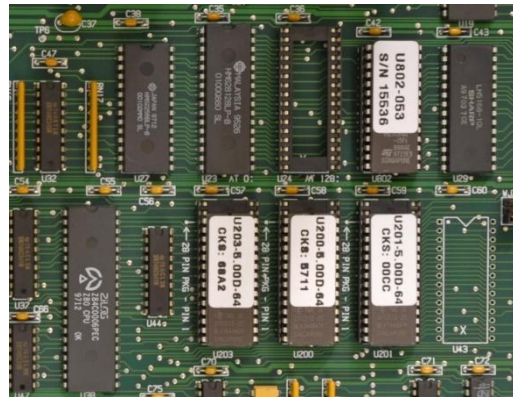
Figure 3: Close-up of ROM chips (with white labels).
