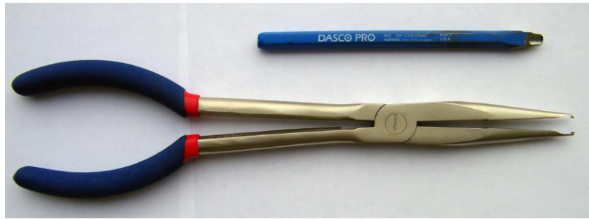
Figure 15: (top) chisel ground to radius of cup; (bottom) pliers ground to grip and remove cap from base
