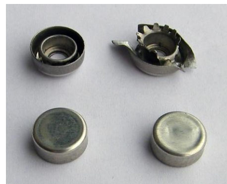
Figure 16: Small cup “seal”. Top left, base; bottom left, cap; top right, base after removal; bottom right, cap after removal
