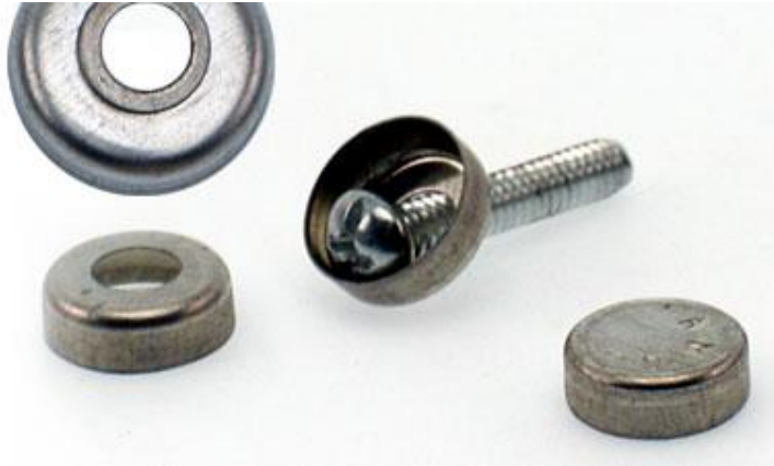
Figure 4 - The American Casting and Manufacturing MCS-C Cup Seal. From reference [31]. The bottom portion of the seal (center, with the screw hole) has a diameter of \sim 0.490'' , while the cap (left and right) has a diameter of \sim 0.464'' .
