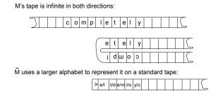
Figure 1.5: To simulate a machine M with alphabet  $\Gamma$  that has tapes infinite in both directions, we use a machine  $\tilde{M}$  with alphabet  $\Gamma^2$  whose tapes encode the "folded" version of M's tapes.
