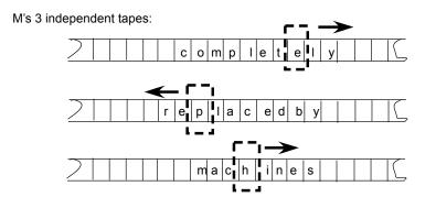
U's 3 parallel tapes (i.e., one tape encoding 3 tapes)
