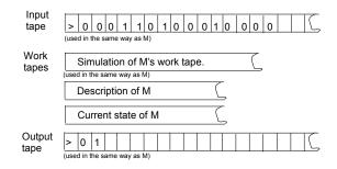
Figure 1.6: The universal TM  $\mathcal{U}$  has in addition to the input and output tape, three work tapes. One work tape will have the same contents as the simulated machine M, another tape includes the description M (converted to an equivalent one-work-tape form), and another tape contains the current state of M.
