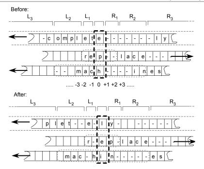
Figure 1.10: Performing a shift of the parallel tapes. The left shift of the first tape involves zones  $L_1, R_1, L_2, R_2, L_3, R_3$ , the right shift of the second tape involves only  $L_1, R_1$ , while the left shift of the third tape involves zones  $L_1, R_1, L_2, R_2$ . We maintain the invariant that each zone is either empty, half-full or full. Note that – denotes  $\Box$ .
