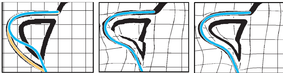
Fig. 16. A variant of “Wires” that removes discontinuities in the warp. Left : Curve features for the warp (closeup). Center : Buckling artifacts caused by discontinuity in the warp. Right : The new warp, with discontinuities removed.
