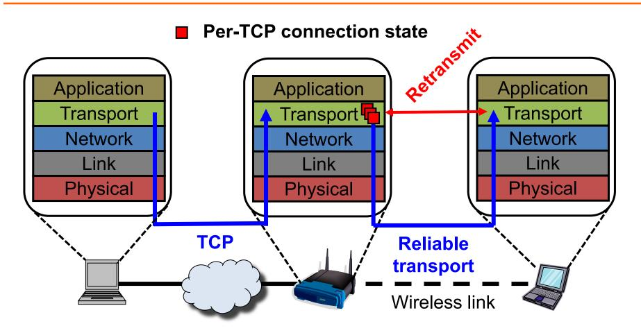
Maintain state for both "halves" of each end-to-end "connection" at the AP
