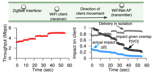
Figure 12: WiFiNet’s ability to track the changing interference patterns for a client that is moving away from a ZigBee interferer. (left) instantaneous throughput at the client (right) delivery in isolation ( i.e. , in absence of overlap), impact given overlap ( p[I|O] ) and actual impact ( p[I] ) are shown.
