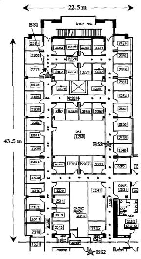
Figure 1 Map of the floor where the experiments were conducted. The black dots denote locations were empirical signal strength information was collected. The large stars show the locations of the 3 base stations. The orientation is North (up) and East (right).
