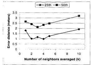
Figure 5 The error distance for the empirical method with averaging on the data set containing the max signal strength measurement for each location.
