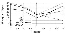
Figure 7: Throughput of a nomadic client at different position between AP1 and AP2 in 802.11n. MPTCP with ECN marking provides 85% of the optimal throughput.
