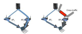
Figure 4: Scenario 1 (left): a client using  $AP_1$  and  $AP_2$  prefers  $AP_2$  because of its more efficient use of airtime. Scenario 2 (right): moving all traffic to  $AP_2$  with its better radio conditions is not the optimal strategy end-to-end
