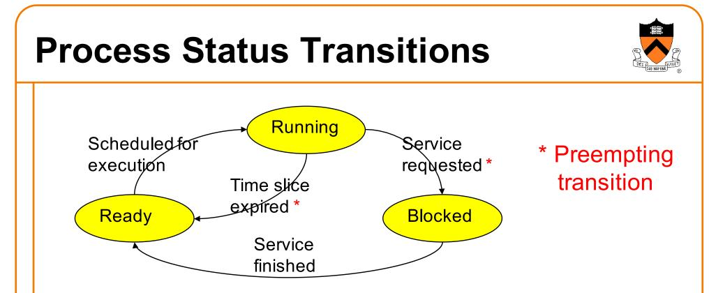
Service requested: OS moves running process to blocked set because it requested a (time consuming) system service (often I/O) Service finished: OS moves blocked process to ready set because the requested service finished Time slice expired: OS moves running process to ready set because process consumed its fair share of CPU time Scheduled for execution: OS selects some process from ready set and assigns CPU to it
